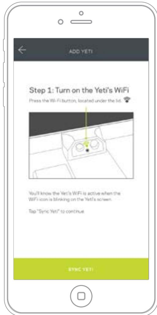
The Yeti's WiFi button is located under the lid. It's the top of the two buttons.
